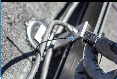
2. Insert cable through open hole.
